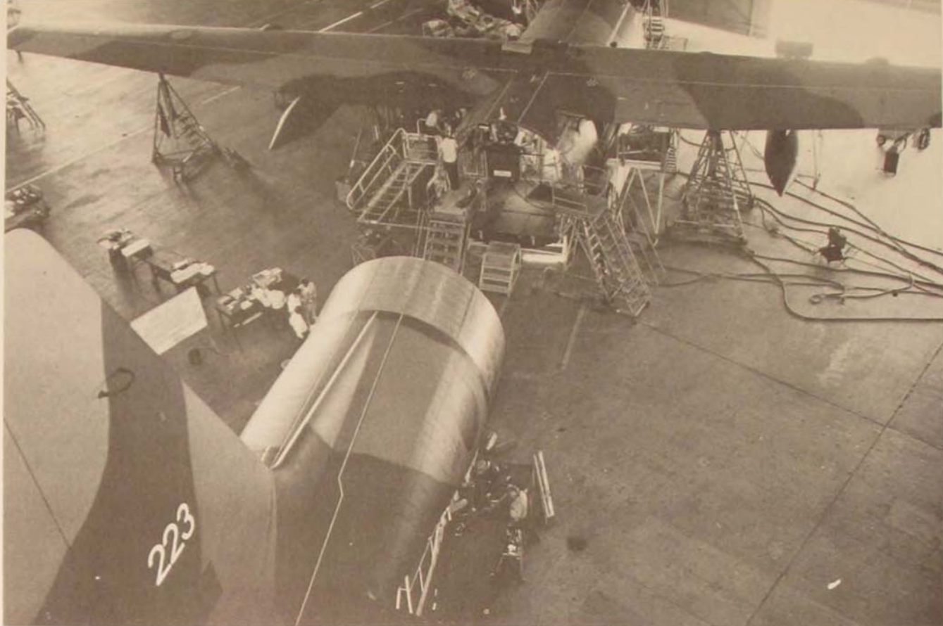
An RAF C-130K undergoes stretch modification. A similar modification to US Air Force C-130s could provide an interim solution until a follow-on tactical airlift aircraft is ready.
